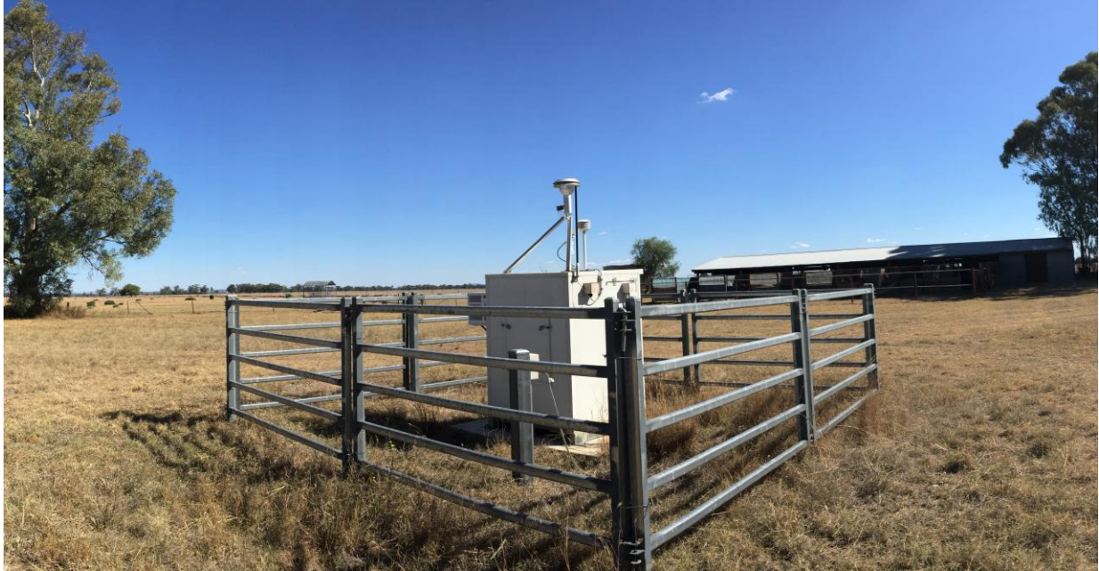
Figure 1: TEOM installed at Flixton property
